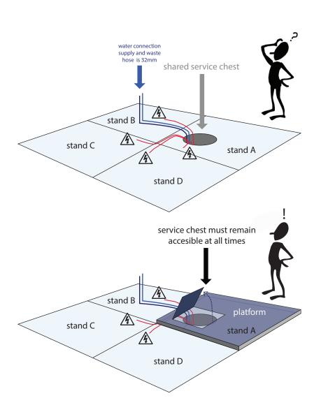
Whenever a service chest is shared between more than one stand in one island, it must remain accessible at all times (through a hatch).
